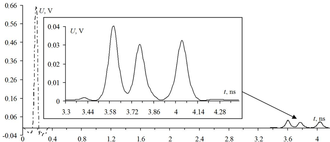
Fig. 3. Waveforms at the input (---) and output (—) (with enlarged fragment of the signal at the output) of three-conductor microstrip line MF with the parameters obtained as a result of heuristic search
