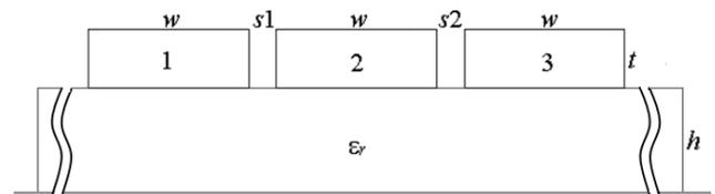
Fig. 2. Cross sections of three-conductor MSL
