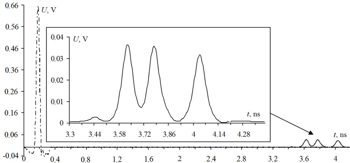
Fig. 6. Waveforms at the input (---) and output (—) (with enlarged fragment of the signal at the output) of three-conductor microstrip line MF after optimization of parameter  $s_1$  using GA
