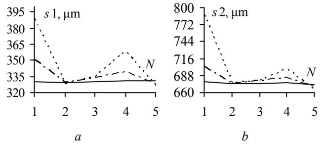
Fig. 5. The results of GA optimization of conductors separations  $s_1$  (a) and  $s_2$  (b) for the number of individuals and generations: 10 and 10 (····); 10 and 30 (-·-·-); 10 and 100 (—)
