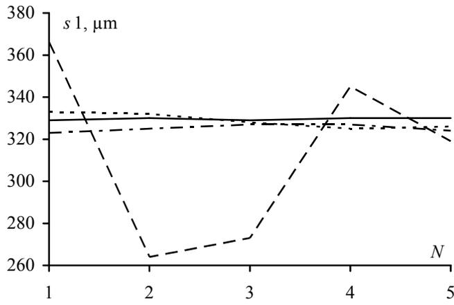
Fig. 4. The results of GA optimization of conductor separation  $s_1$  for the number of individuals and generations: 3 and 10 (---); 10 and 10 (····); 10 and 30 (-·-·-); 10 and 100 (—)
