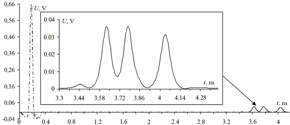
Fig. 7. Waveforms at the input (---) and output (—) (with enlarged fragment of the signal at the output) of three-conductor microstrip line MF after optimization of parameters  $s_1$  and  $s_2$  using GA
