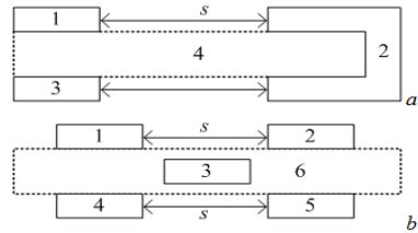
Fig. 1. Cross section of the examined structures: 1 – symmetrical MF with broad-side coupling (1–3 – conductors, 4 – dielectric) (a); 2 – reverse symmetrical MF (1–5 – conductor, 6 – dielectric) (b)
