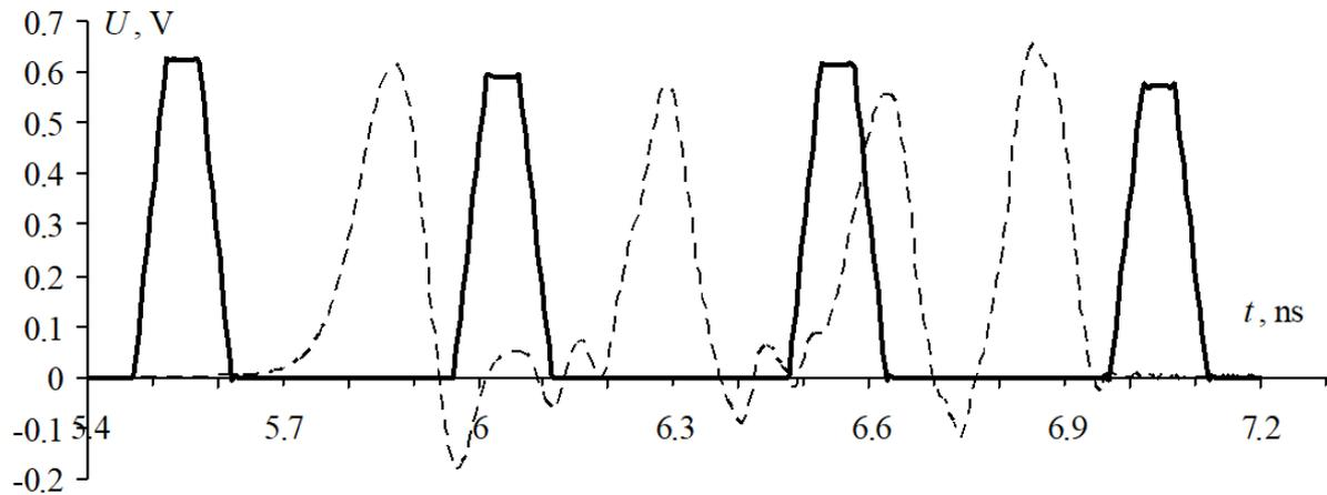
**Figure 2.** Voltage waveforms at the output of reflection symmetric MF under quasi-static (—) and electrodynamic (---) analysis without taking into account the losses.
