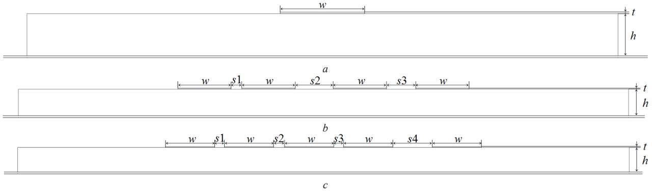
Fig. 1. Cross sections of one- (a), four- (b) and five- (c) conductor MSL
