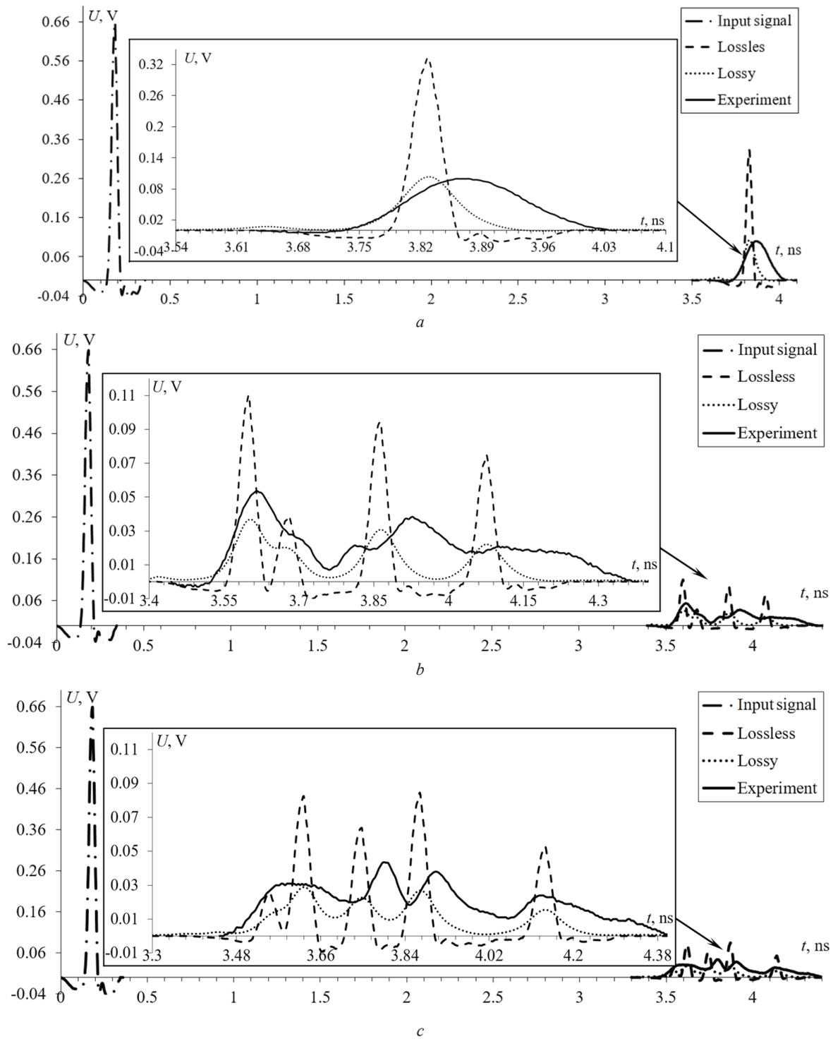
Fig. 4. Waveforms of signal at the input (---) and output (with their enlarged fragments) single- (a), four- (b) and five-conductor (c) MSL, resulting from the simulation excluding (---) and including (····) losses, via experiment (—)
