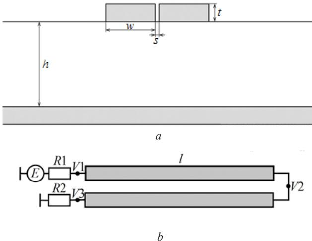
Fig. 1. Cross section (a) and scheme (b) of the meander microstrip line
