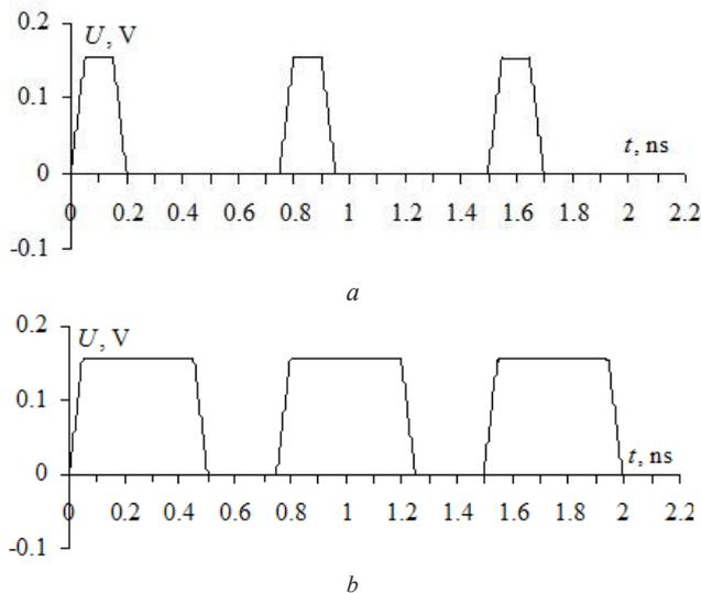
Fig. 4 Waveforms at the output of investigated line with the duration of impact pulses 200 (a) and 500 ps (b), fulfilled condition (3) and the additional optimization
