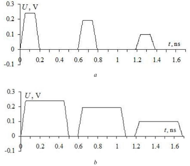
Fig 3 Waveforms at the end of investigated line with the excitation pulses duration of 200 (a) and 500 ps (b) and fulfilled condition (3)
