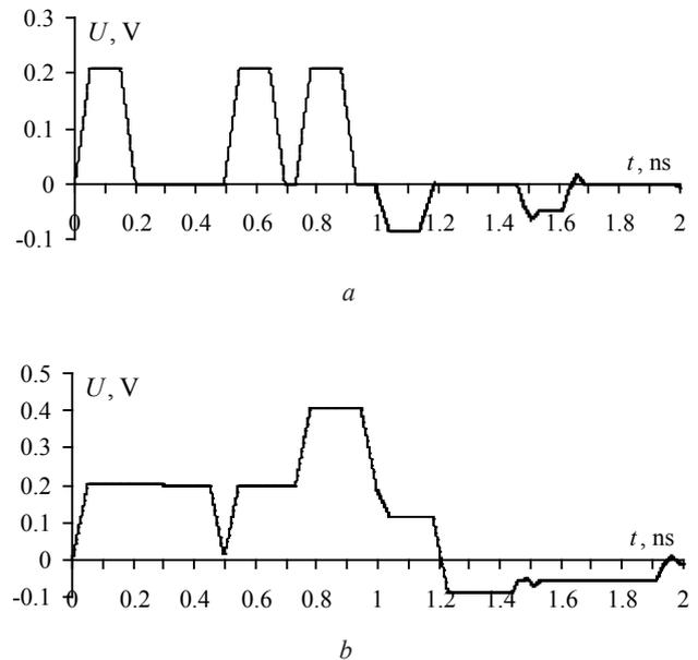
Fig. 2 Waveforms at the end of investigated line with the excitation pulses duration of 200 (a) and 500 ps (b)
