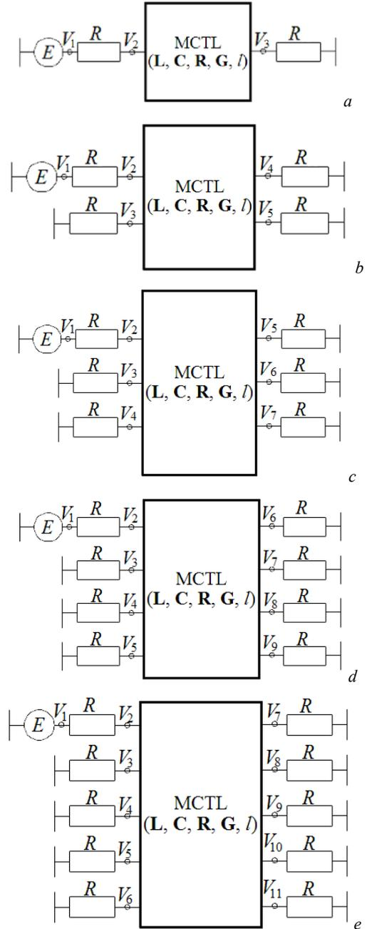
Fig. 2. Schematic diagrams of one- (a), two- (b), three- (c), four- (d) and five-conductor (e) MFs
