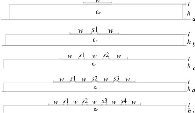
Fig. 1. Cross sections of one- (a), two- (b), three- (c), four- (d) and five-conductor (e) MFs
