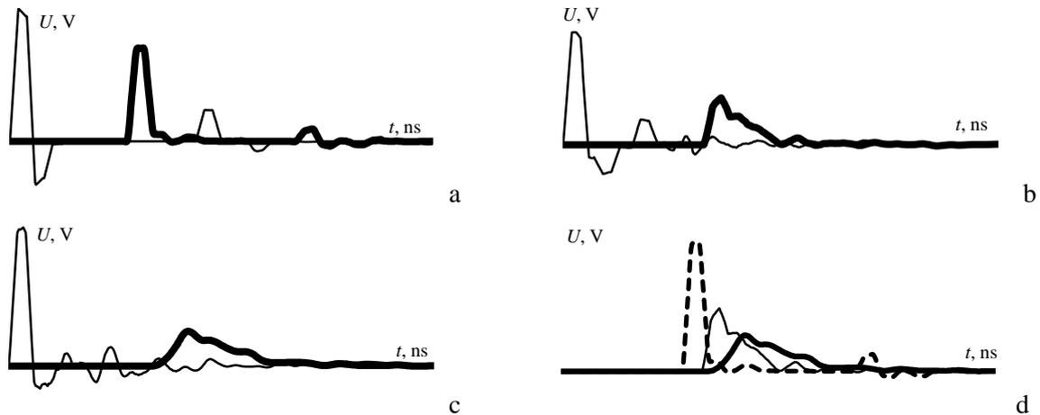
**Figure 7.** Voltage waveforms at near and far ends of the line for PCB: a – without modal reservation; b – with modal reservation when  $\epsilon_r = 4.2$ ; c – with modal reservation when  $\epsilon_r = 10$ . Comparison of waveforms (d) at the far end without modal reservation (---) and with modal reservation when  $\epsilon_{r2} = 4.2$  (—) and  $\epsilon_{r2} = 10$  (—).
