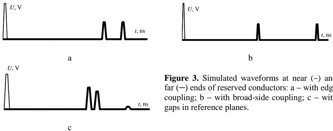
**Figure 3.** Simulated waveforms at near (–) and far (–) ends of reserved conductors: a – with edge coupling; b – with broad-side coupling; c – with gaps in reference planes.
