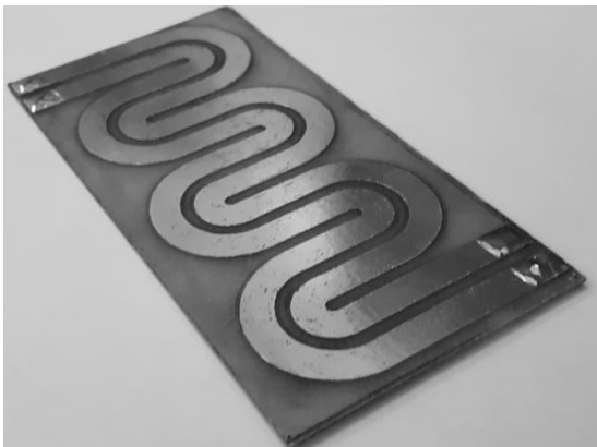
Fig. 6. The prototype of the MF PCB: top (a), and bottom(b) views.
