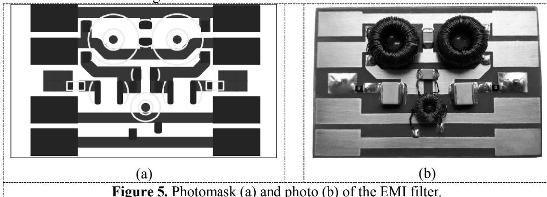
**Figure 5.** Photomask (a) and photo (b) of the EMI filter.
