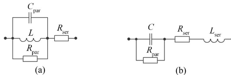
**Figure 3.** Equivalent circuits of a choke (a) and a capacitor (b).
