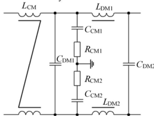
**Figure 1.** Schematic diagram of the developed filter.
