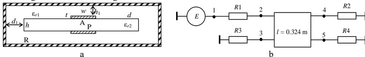
**Figure 1.** Cross section (a) and schematic diagram (b) of a structure with single MR in the TALGAT system where conductors – active (A), passive (P), and reference (R).
