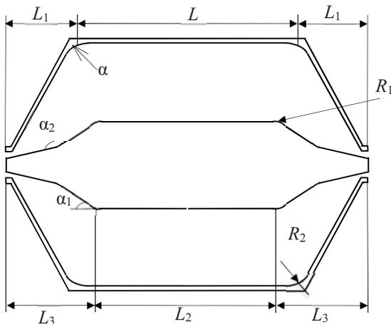
Fig. 6. Longitudinal section of the TEM cell model with a tapering enclosure width at a constant height.
