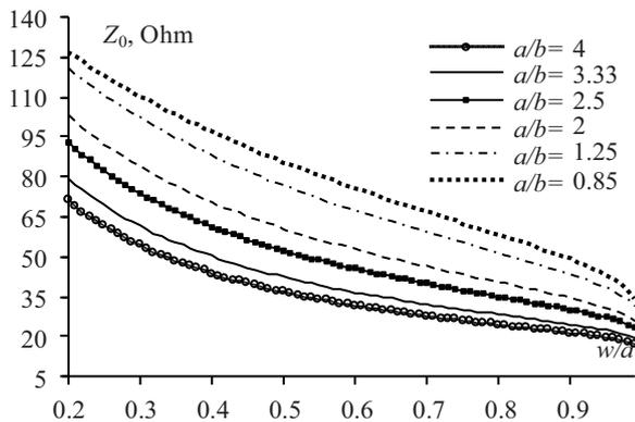
Fig. 2. Dependences of the characteristic impedance  $Z_0$  on the ratio  $w/a$  for different  $a/b$ .
