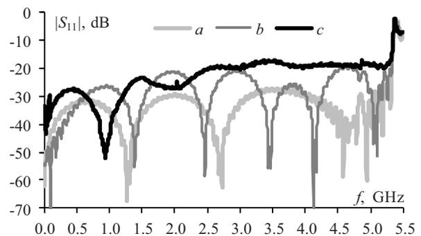
Fig. 12. Frequency dependencies of  $|S_{11}|$  for electrodynamic (a), solid (b) models and the research prototype (c) of the TEM cell.
