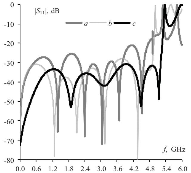
Fig. 7. Frequency dependences of  $|S_{11}|$  of TEM cell models with pyramidal transitions (a), rectangular enclosure (b), tapering transitions at a constant height of the enclosure (c).
