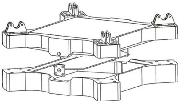
Fig. 9. Isometric view of a solid model of the TEM cell.
