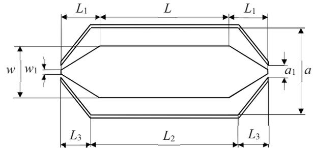
Fig. 4. Longitudinal section of the TEM cell model with pyramidal transitions.
