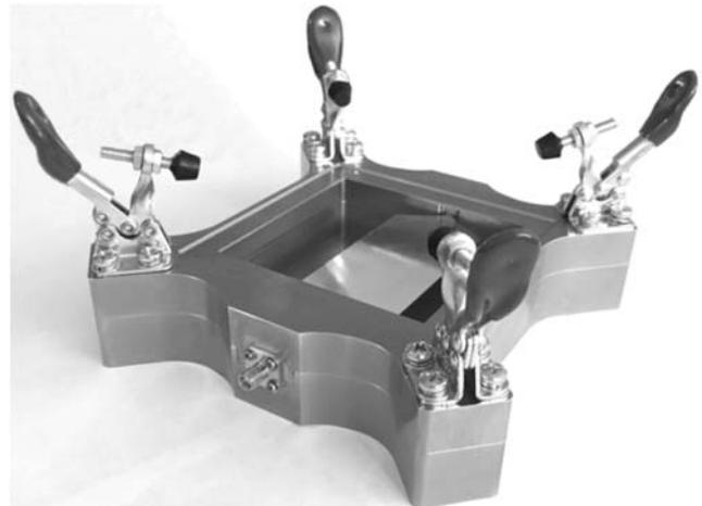
Fig. 10. The research prototype of the TEM cell without a test table.
