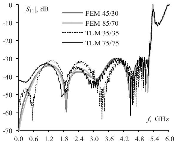
Fig. 8. Frequency dependencies of  $|S_{11}|$  of the TEM cell models obtained using the TLM and FEM with reduced mesh size.
