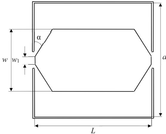
Fig. 5. Longitudinal section of the TEM cell model with a rectangular enclosure.
