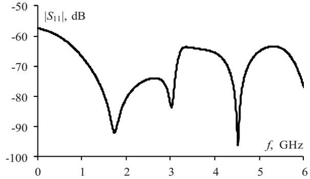
Fig. 3. Frequency dependence of  $|S_{11}|$  of the regular part of the TEM cell.
