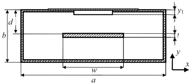
Fig. 1. Cross-section of TEM cell with the DUT.
