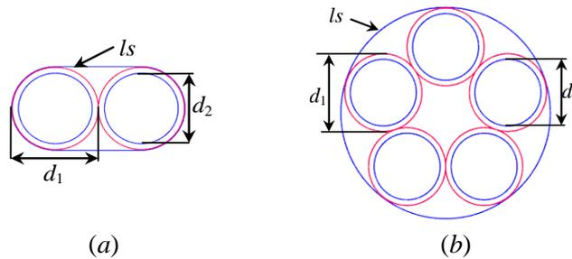
**Figure 3.** The cross-sections of central (sections 3, 4, 15, 16 – *a*) and side (sections 1, 2, 5, 6, 13, 14, 17, 18– *b*) branches.
