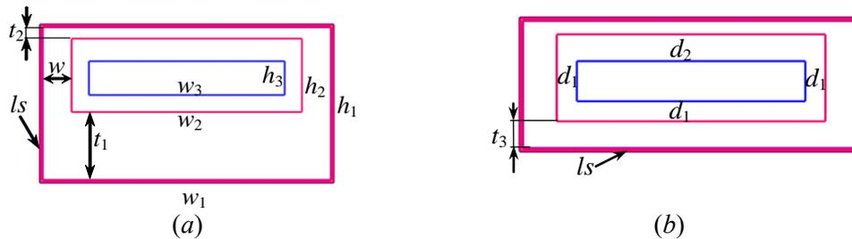
**Figure 2.** The cross-sections of big part (sections 7 and 12 – *a*) and the small part (sections 8–11 – *b*) of the PS bus.
