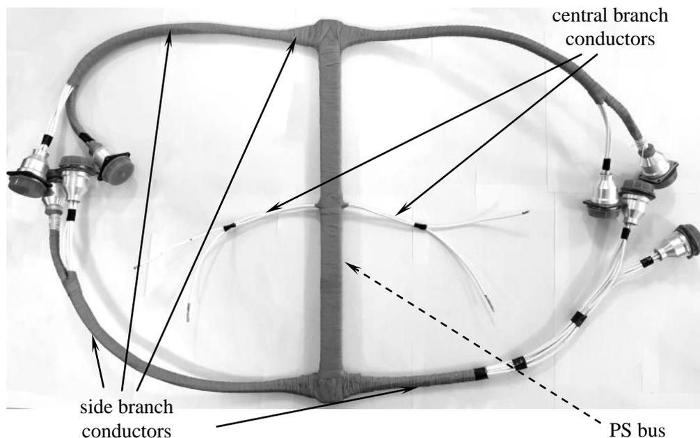
**Figure 1.** The photo of the experimental model.
