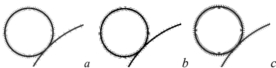
Fig. 4. Conductor segmentation: 100 (a), 200 (b) and 300 (c) intervals
