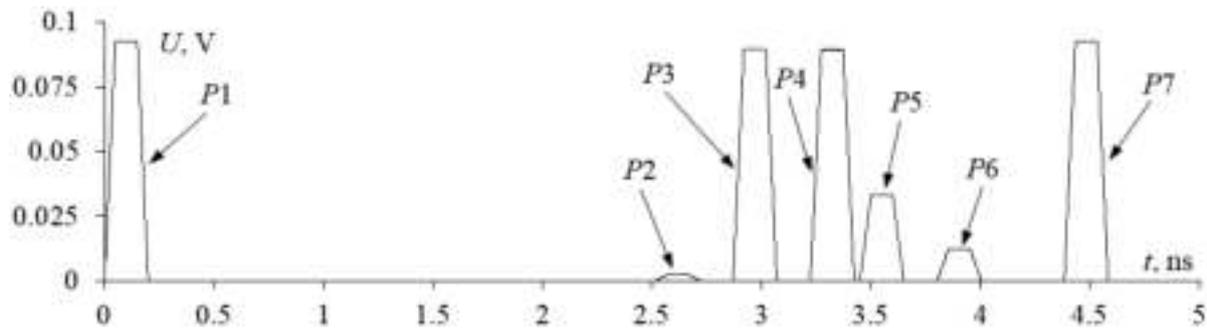
**Figure 4.** Voltage waveform at node  $V_4$  at optimal geometric line parameters which ensure the fulfillment of conditions (7)–(10)
