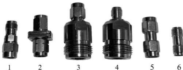
Fig. 7. Coaxial adapters used in the experiment.
