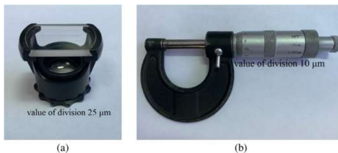
Fig. 5. Magnifying glass with a measuring ruler (a) and a mechanical micrometer (b).
