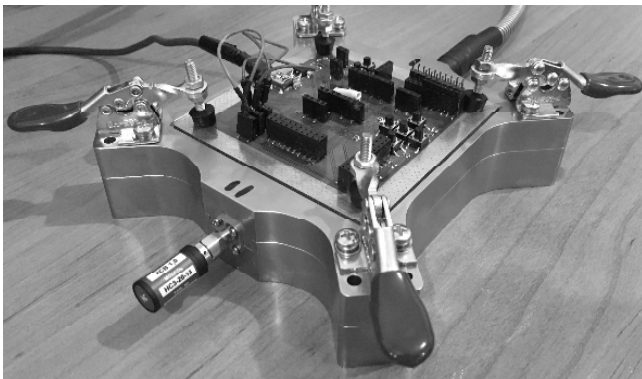
Fig. 2. Setup for testing radiated emissions of ICs in a TEM cell
