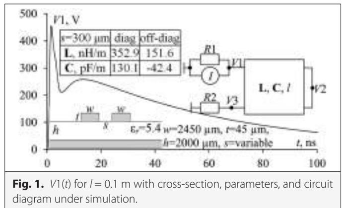
**Fig. 1.**  $V_1(t)$  for  $l = 0.1$  m with cross-section, parameters, and circuit diagram under simulation.
