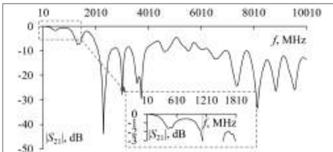
Fig. 11. Measured frequency dependence of  $|S_{21}|$  for the meander MSL prototype with  $s = 150 \mu\text{m}$  and  $l = 90 \text{ mm}$  from [17].
