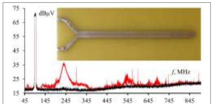
Fig. 13. Measured voltage spectra at the outputs of the modulator (—) and the turn (—) with a carrier frequency of 96 MHz, and photo of meander MSL prototype with  $s = 150 \mu\text{m}$  and  $l = 90 \text{ mm}$  from [17].
