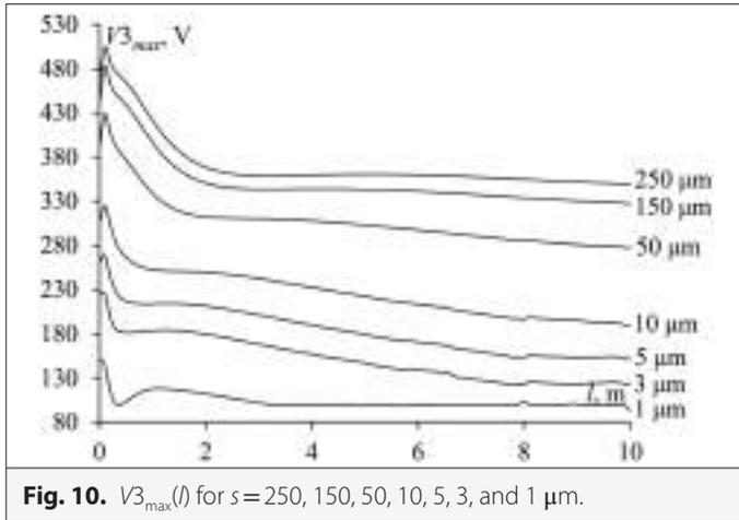
Fig. 10.  $V_{3_{max}}(l)$  for  $s = 250, 150, 50, 10, 5, 3,$  and  $1 \mu\text{m}$ .
