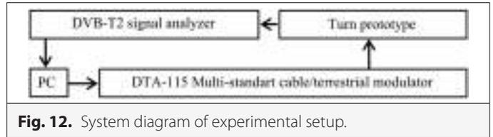
Fig. 12. System diagram of experimental setup.
