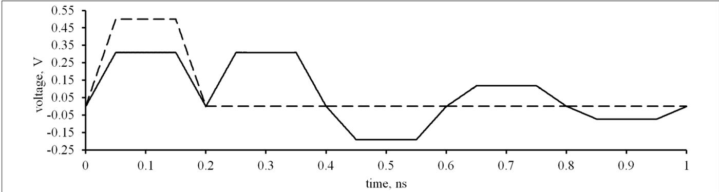
**Fig. 4.** Voltage waveforms at nodes  $V_1$  (---) and  $V_2$  (—) of the ML in the air filling when  $k \approx 4.236$ .
