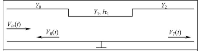
Fig. 2. Equivalent circuit of the transmission line segment with terminations.
