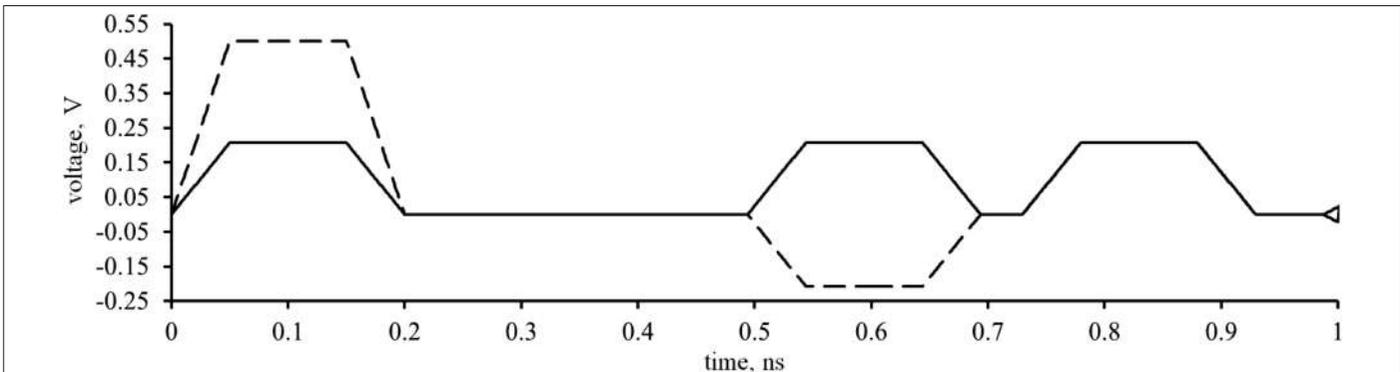
**Fig. 5.** Voltage waveforms at nodes  $V_1$  (---) and  $V_2$  (—) of the microstrip ML turn when  $k \approx 2.413$ .
