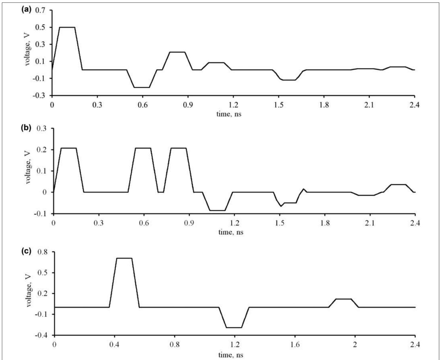
**Fig. 3.** Voltage waveforms at nodes  $V_1$  (a),  $V_2$  (b), and  $V_3$  (c) of the circuit in Fig. 1 calculated using expressions (12–14) (–) and with TALGAT.
